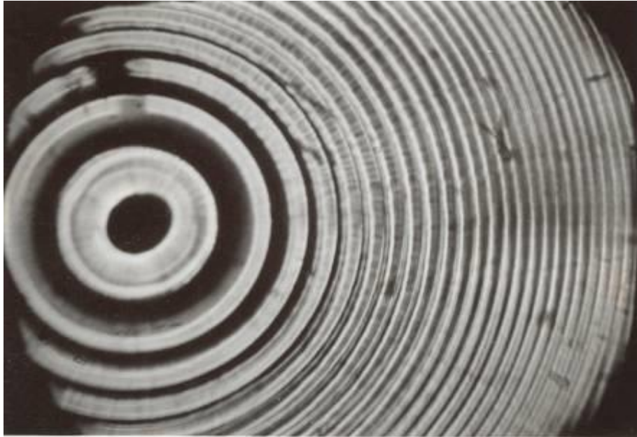
Microphoto of cross section of produced preform
