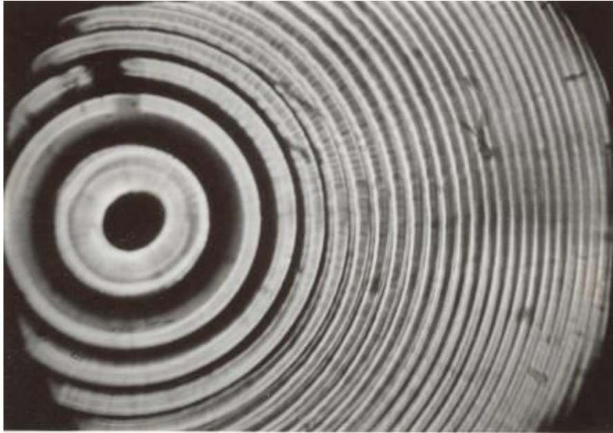
Microphoto of cross section of produced preform
